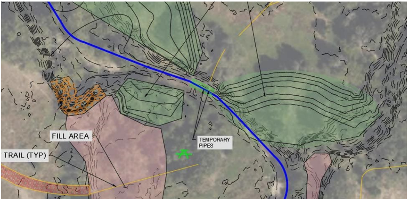
Figure 39: Temporary pipes used during construction.
